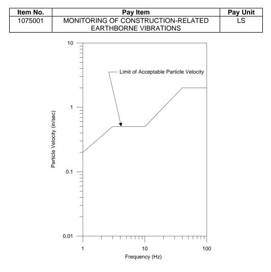
Figure 1 - Vibration Criteria (adapted from AASHTO R8-96)
